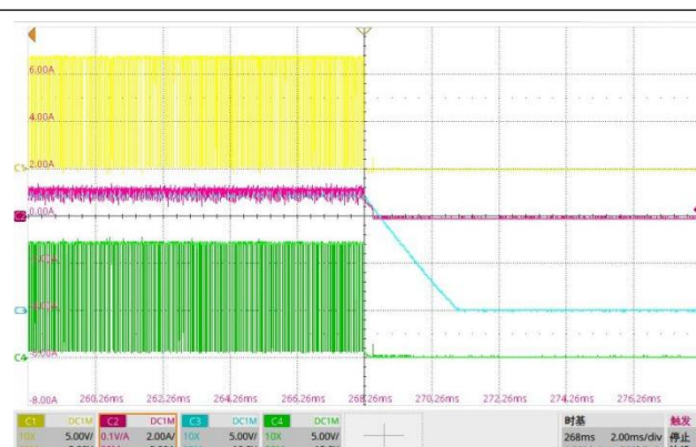
Fig. 8-14 Steady State waveform, Iout=3A
