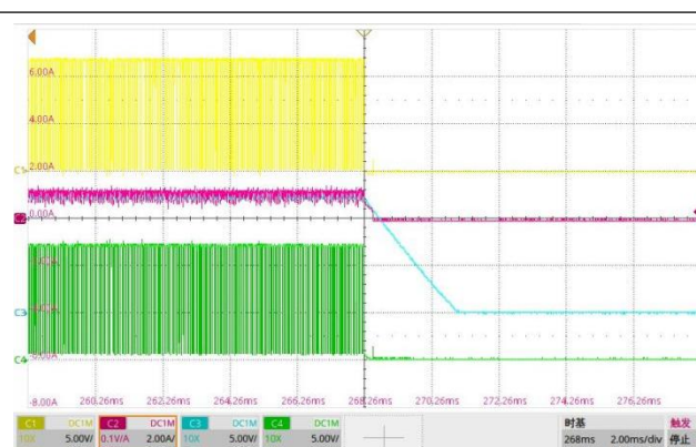
Fig. 8-14 Steady State waveform, Iout=3A
